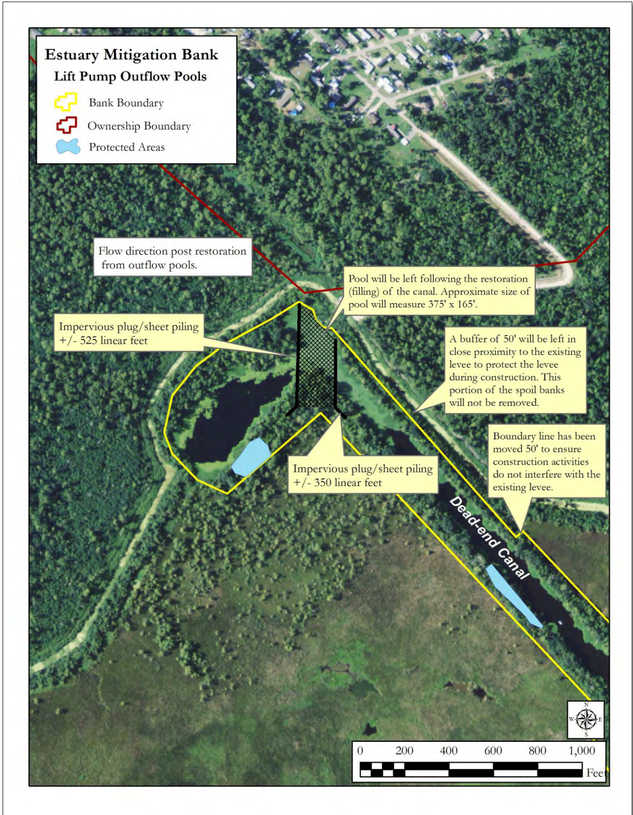
Figure 6b. Close up of outlet pool. Water will exit the pool to the south into the existing marsh.
